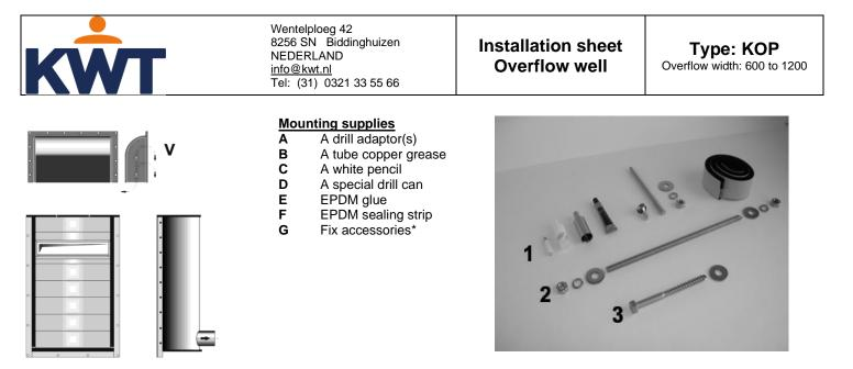
Fix: \*2 - Wood with through hole studs. Holes 2 mm larger than stud diameter. \*3 - Wood with coach screws.
